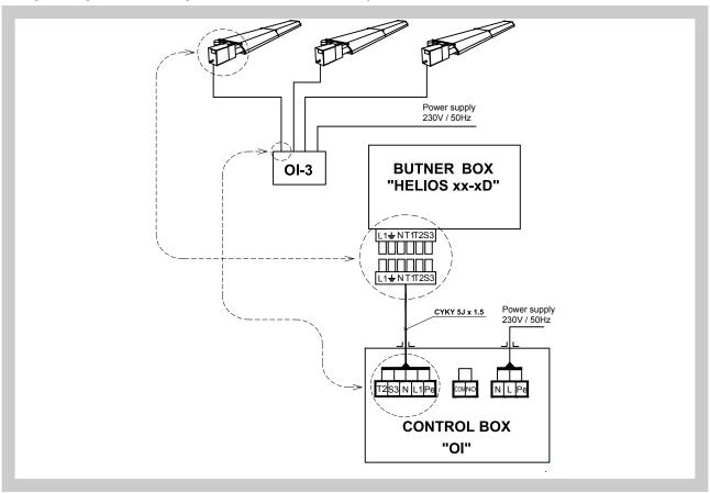
Fig. 16 Diagram of controlling the infrared heater HELIOS-S by control box OID
