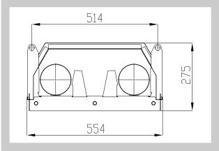
Fig. 2 Reflestor cross section of HELIO SI(D)+
