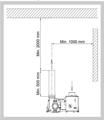
The flue gas exhaust is forced by the flue gas duct inside the building. The appliance is classified according to the flue into design version A<sub>2</sub>. The design and installation of the flue gas exhaust must comply according the correct norm.
