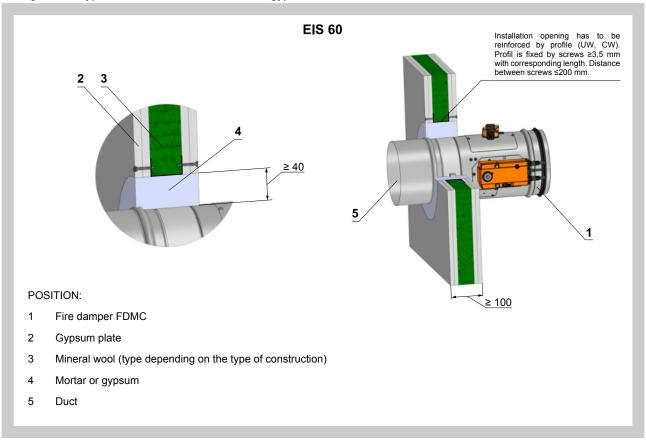
Fig. 21 Gypsum wall construction - stuffing box and fire protection mastic
