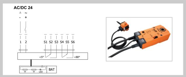
Tab. 2.1.1. Actuating mechanism BELIMO BFL 24-T(-ST), BFL 230-T
