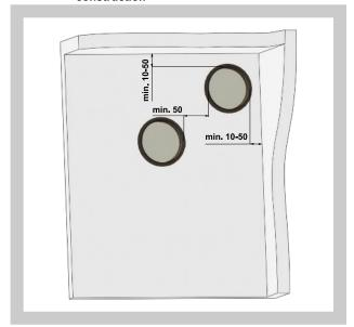
Fig. 12 Built-in edge - design with outer mechanical control or actuating mechanism
