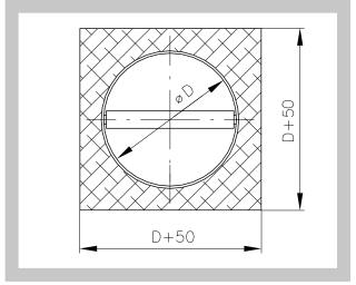
Fig. 14 Installation opening
