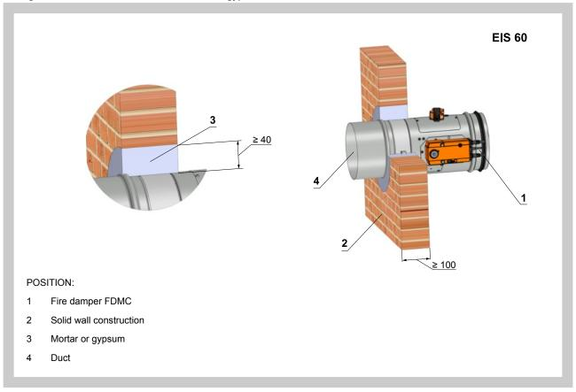
Solid wall construction - stuffing box and fire protection mastic
