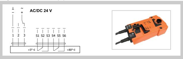
Fig. 7 Actuator BELIMO BEE 24-SR
