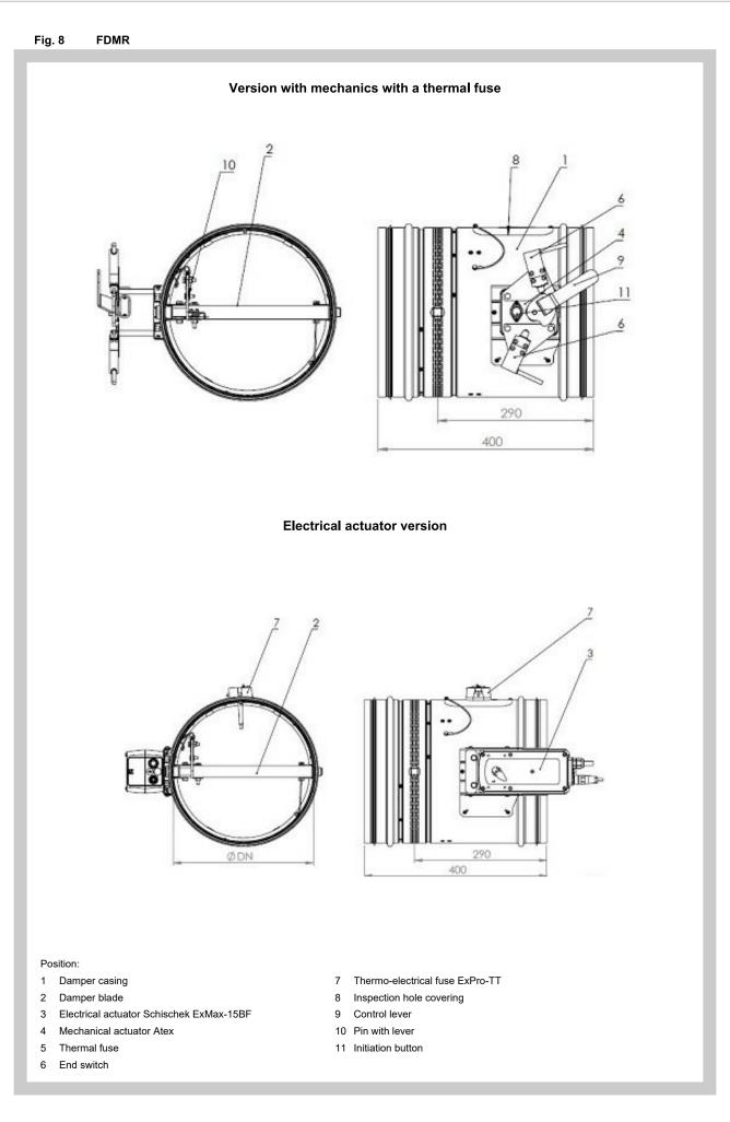
**4.1.** Square dampers are manufactured in the size range (A x B): from 150 x 150 mm to 1500 x 800 mm. Circular dampers: from a diameter of 100 mm to 1000 mm.
