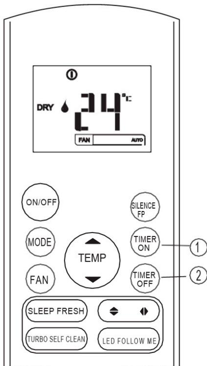
Press the **TIMER ON** button can set the auto-on time of the unit. Press the **TIMER OFF** button can set the auto-off time of the unit
