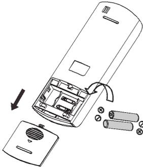
The remote controller is powered by two dry batteries (R03/LR03X2) housed in the back rear part and protected by a cover.
