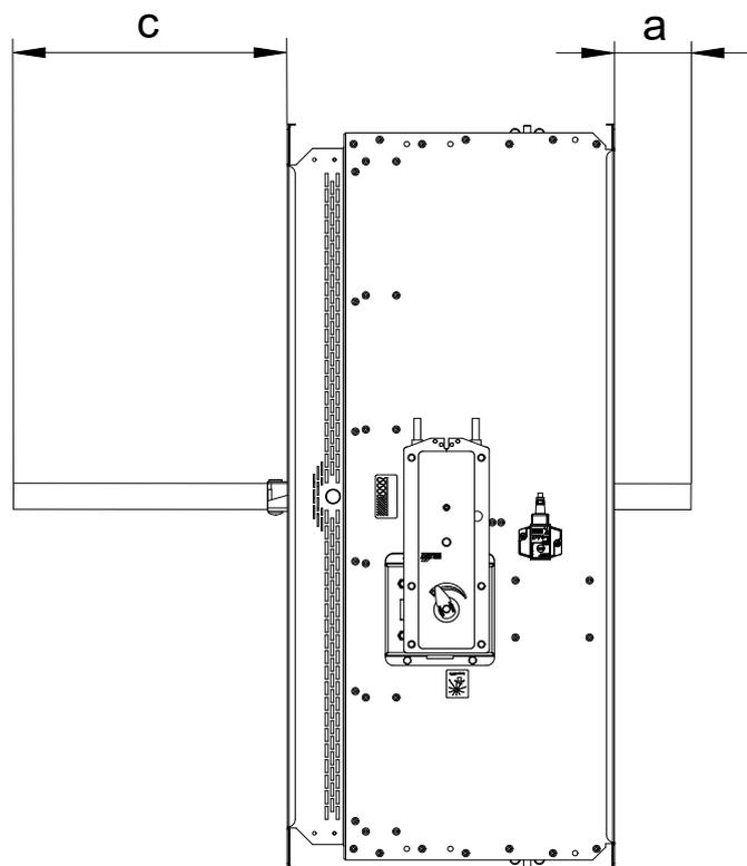
Values "a" and "c" has to be respected when projecting related air-conditioning ducts.
