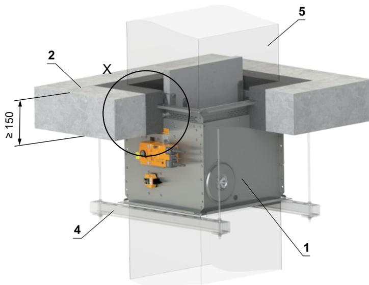
\* In the case of fire resistance EI 120, the installation gap is limited to 50 mm <sup>+10/-0</sup>.
