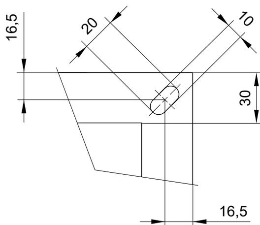
**Flange of a damper - INSTALLATION SIDE**
