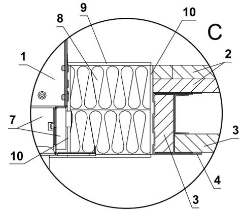
\* In the case of fire resistance EI 90, the installation gap is limited to 90 mm <sup>+0/-10</sup>. For fire resistance EI 60 or lower, an installation gap range of 40–130 mm is permitted.
