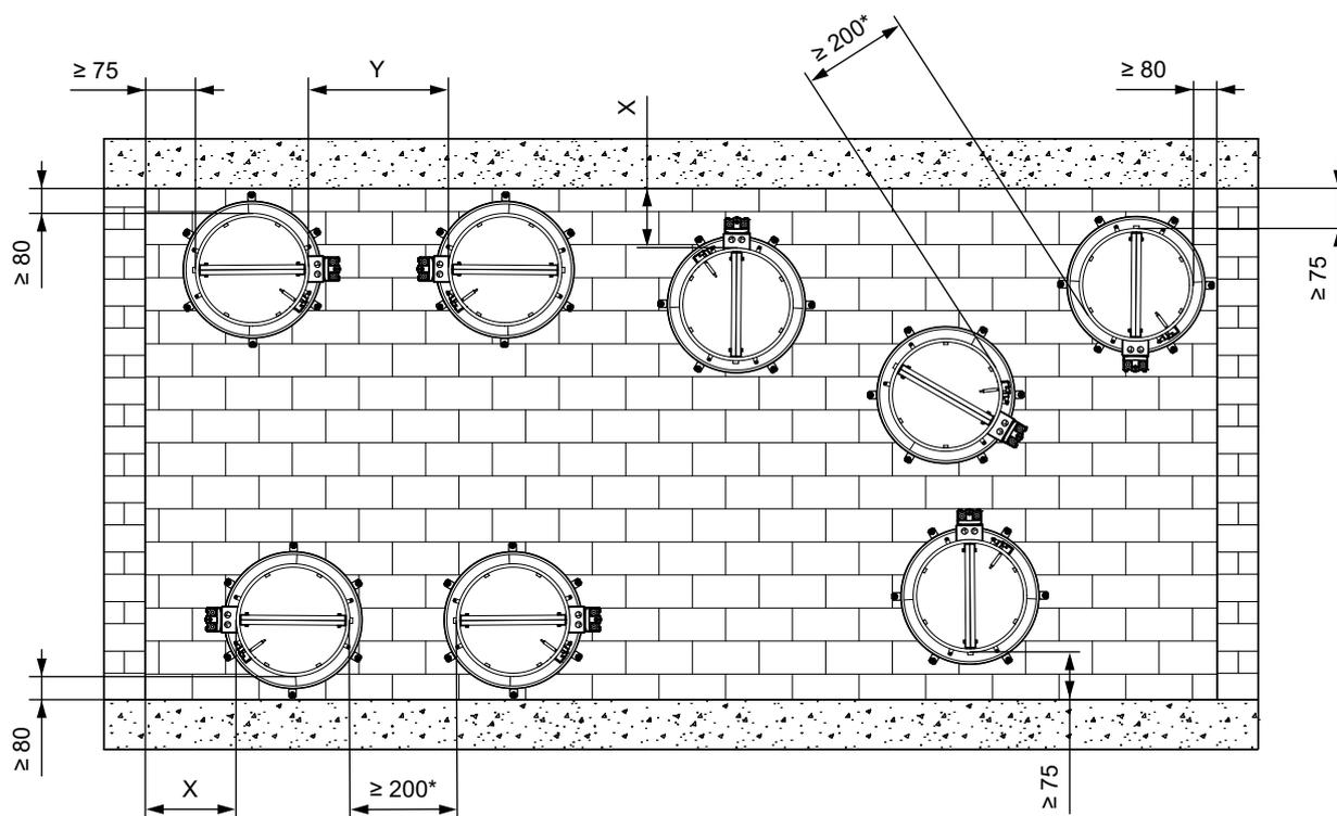
X = recommended min. distance  $\geq 220$  mm required to access the actuator or manual control
