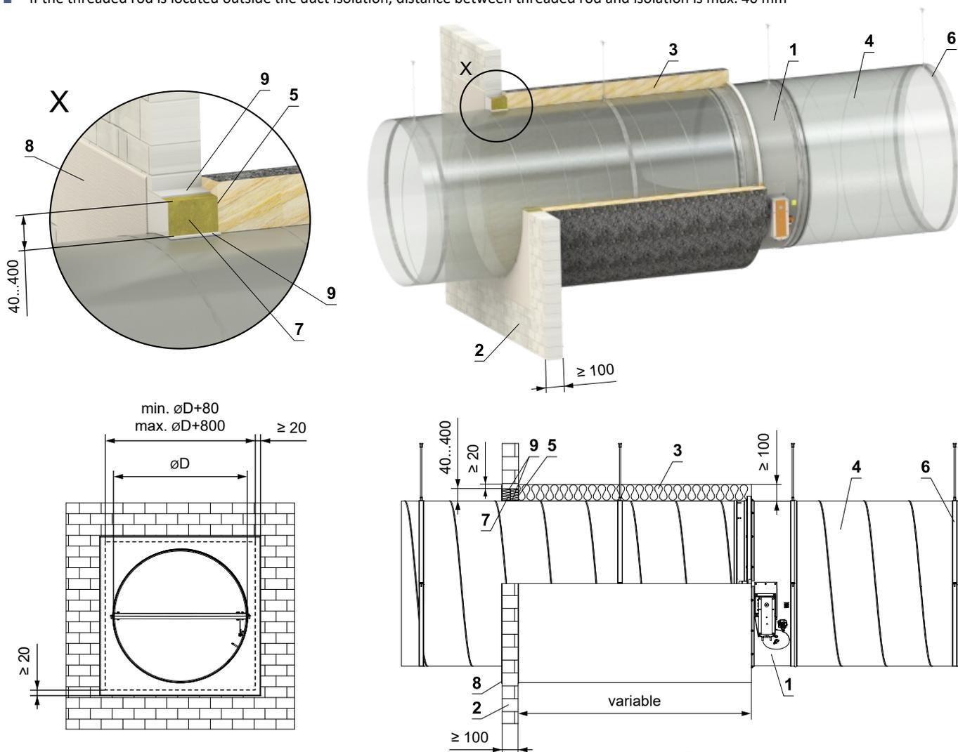
\* HILTI system can be replaced by a similar system with the same or higher thickness, density, fire reaction class, tested according to EN 1366-3.
