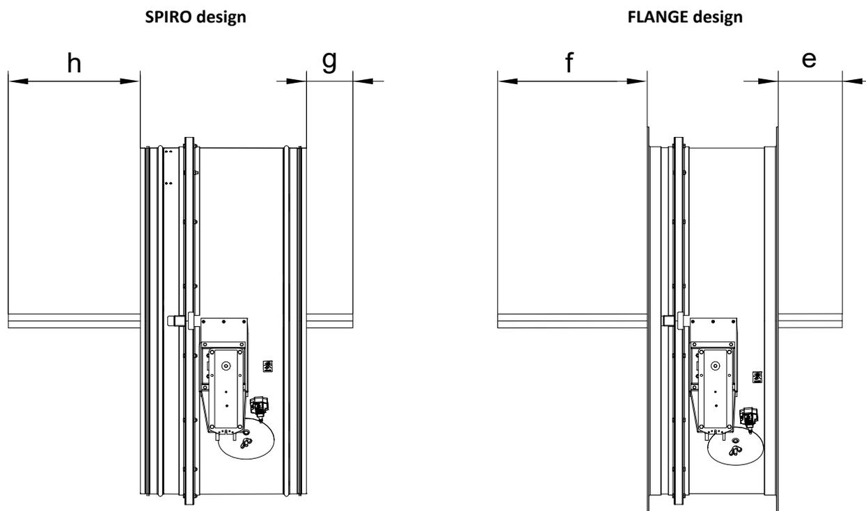
Values "h" and "g" resp. "f" and "e" has to be respected when projecting following air-conditioning duct.
