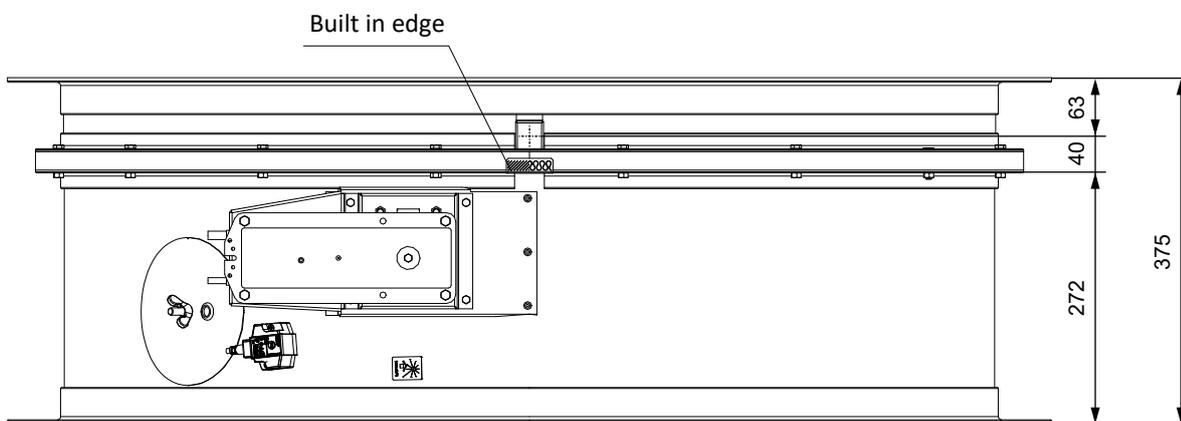
Dimensions of an installation opening
