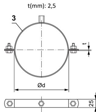
2x screw connection M10x30 or threaded rods M10
