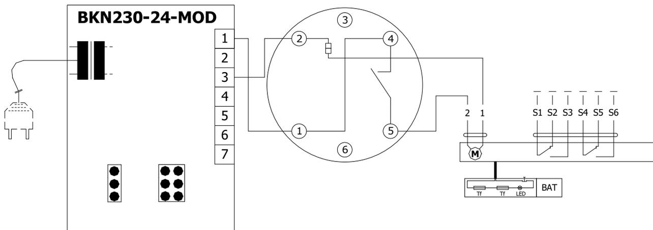
**Design .51 with actuator BF 24-TN (BFL, BFN 24-T), with smoke detector ORS 142 K (voltage 24 V DC)**
