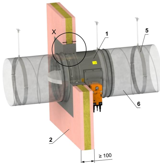
\* In the case of fire resistance EI 120, the installation gap is limited to 50 mm <sup>+10/-0</sup>.
