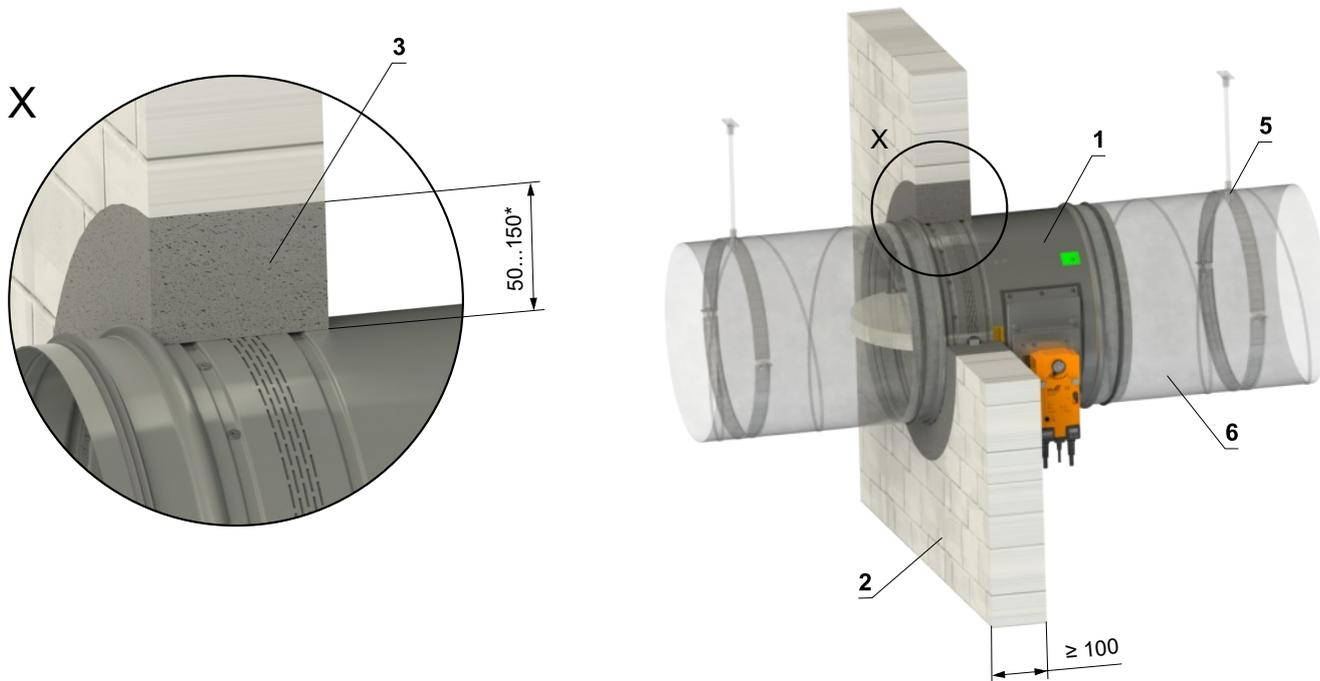
\* In the case of fire resistance EI 120, the installation gap is limited to 50 mm <sup>+10/-0</sup>.
