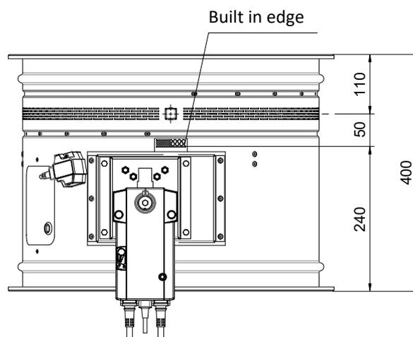
Dimensions of an installation opening
