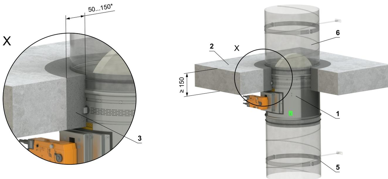
\* In the case of fire resistance EI 120, the installation gap is limited to 50 mm <sup>+10/-0</sup>.
