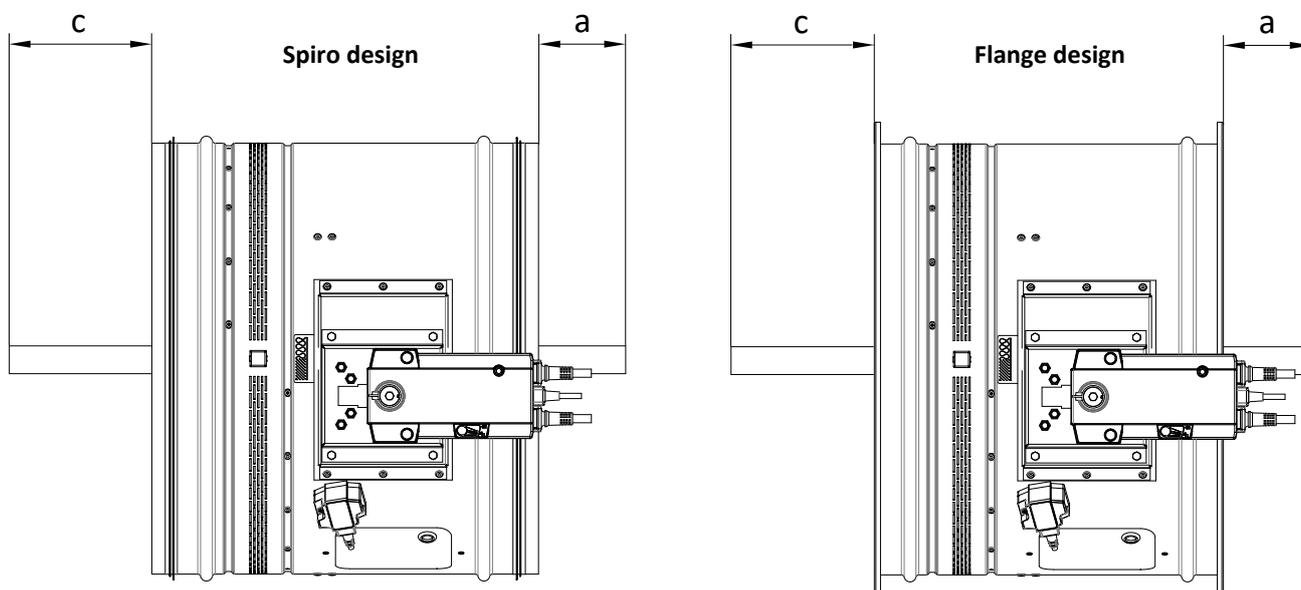
Values "a" and "c" has to be respected when projecting following air-conditioning duct.
