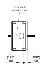
\*Crucial that damper actuator access cover can be removed once fire stop is completed.
