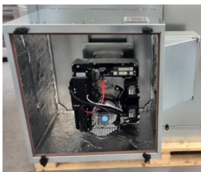
Figure 26 Inner installation of Pecín gas burner
