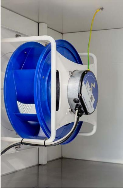
The air is conveyed by means of impellers with the blades that are bent backwards; the impellers are propelled by EC/AC electric motors.
