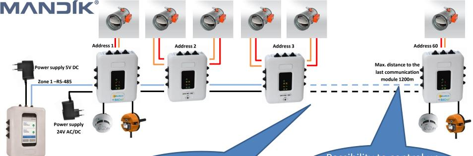
Max. distance can be extended by another 1200m using a repeater
