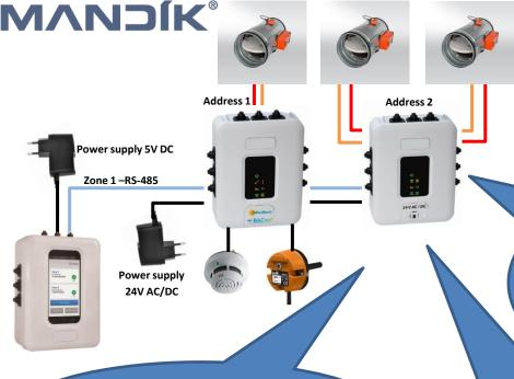
Possibility of connection both dampers through the cable or through AMP-plug
