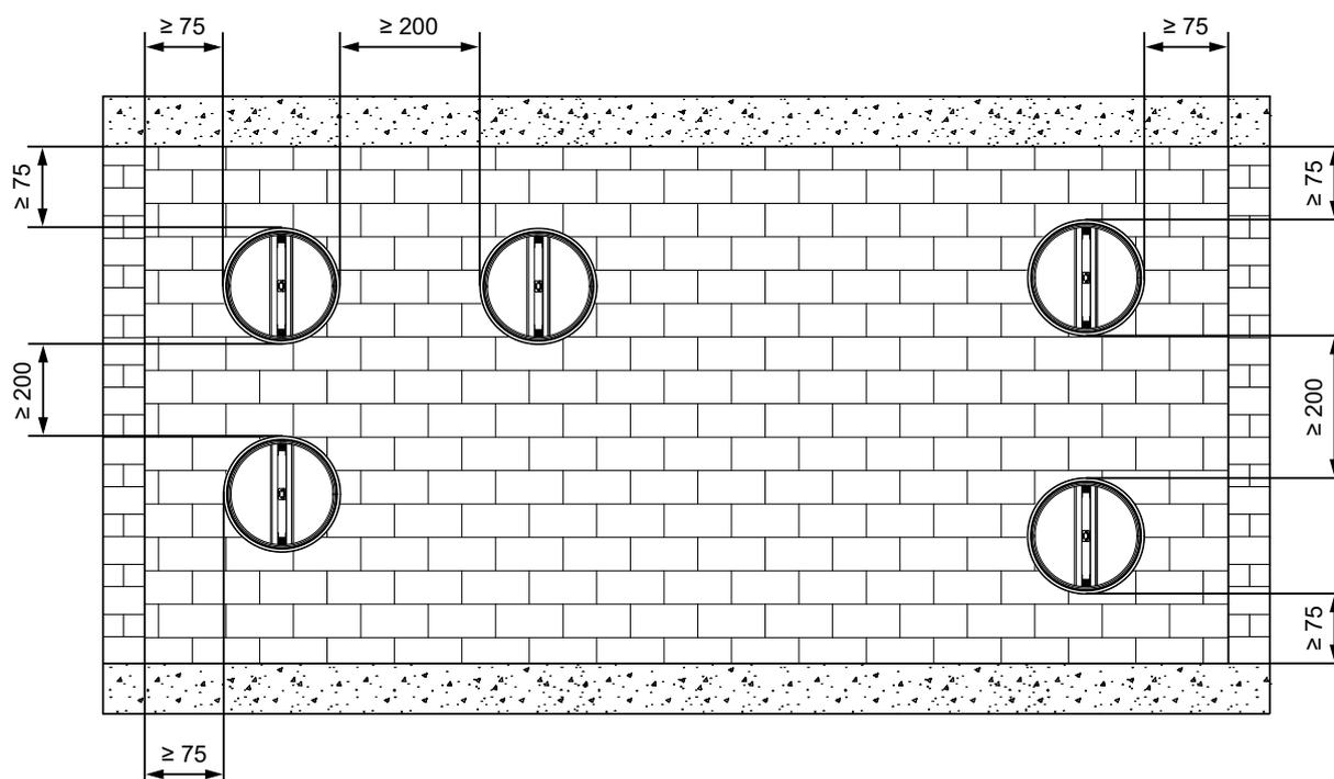
Dimensions of an installation opening
