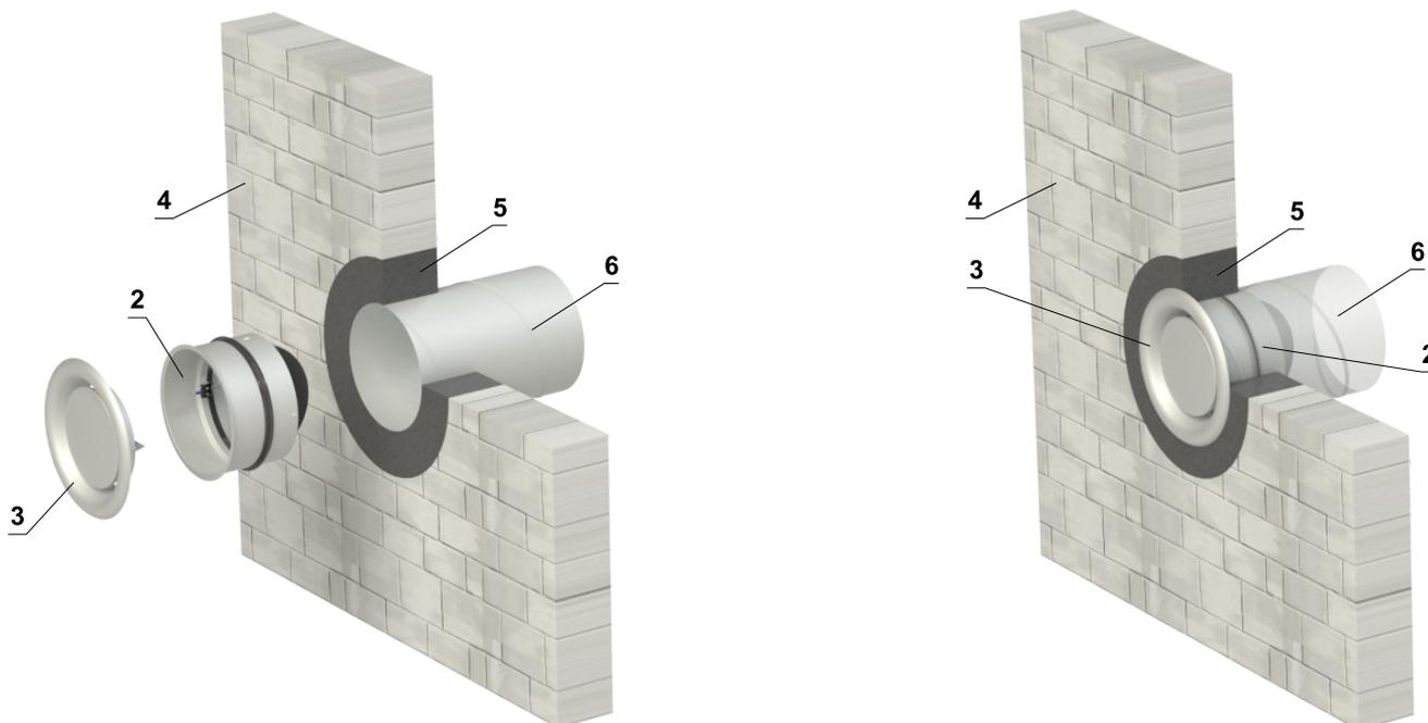
Installation procedure of the CFDM-V damper
