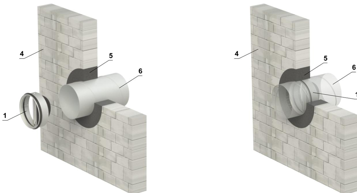
Installation procedure of the CFDM damper
