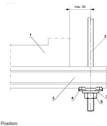
Drop rod and hanger position is not critical and can be positioned to suit the
