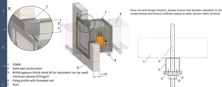
FDMB can be installed with blade axis positioned either vertically or horizontally and with the actuator positioned at 0°, 90° or 270°, but not at 180°
